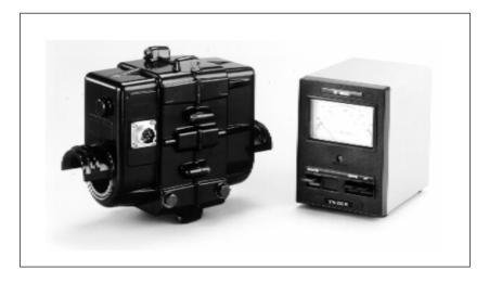
The Yaesu G-550 provides 180° elevation control of unidirectional satellite antenna arrays under remote control from the station operating position. The factory-lubricated rotator unit is housed in weatherproof melamine resin coated die-cast aluminum, to provide maintenance-free operation under all climatic conditions.
